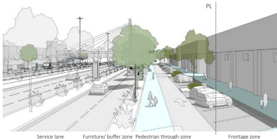
Figure 135 Example of correct organization of pedestrian environment for a main access corridor
