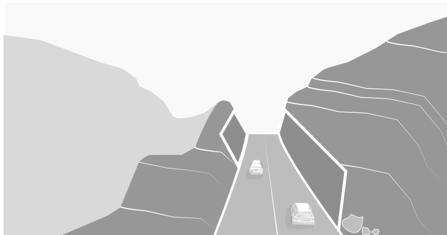
Figure 117 Rectilinear road alignment with cuts, fills and retaining walls have a strong negative environmental and visual impact
