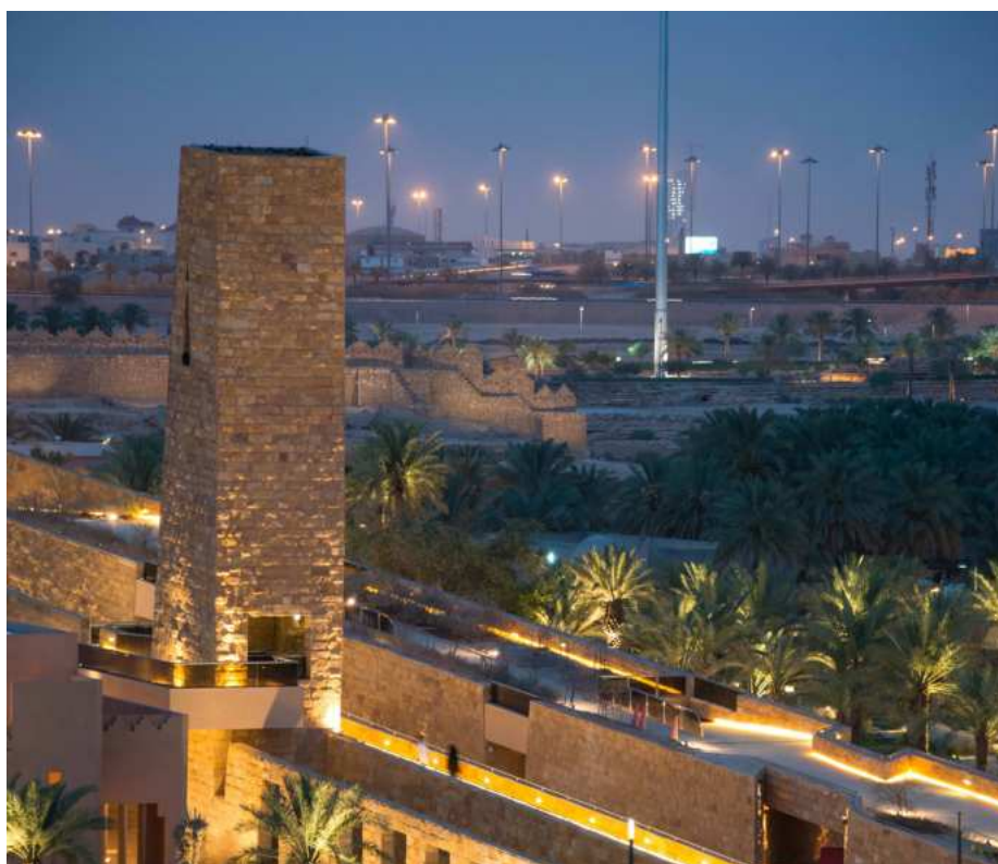
Lighting design with shielded lights, uplighting and highlighting facade features and landscape lighting
