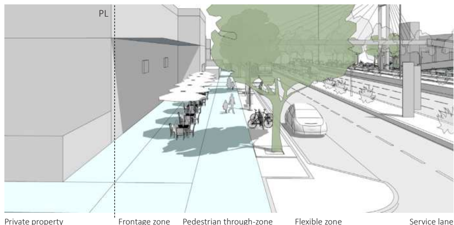
Figure 134 Example of correct organization of pedestrian environment for a main access corridor
